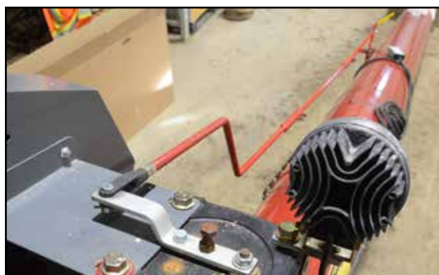
Fig 53 - Rod and linkage installed
